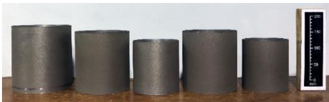
Figure 2 All completed PBF shell specimens (with decreasing slenderness from left to right)
