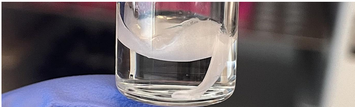
Figure 17. Film formation of a control-A-PLGA sample at the interface of air and PBS, while remaining strip under the interface.
