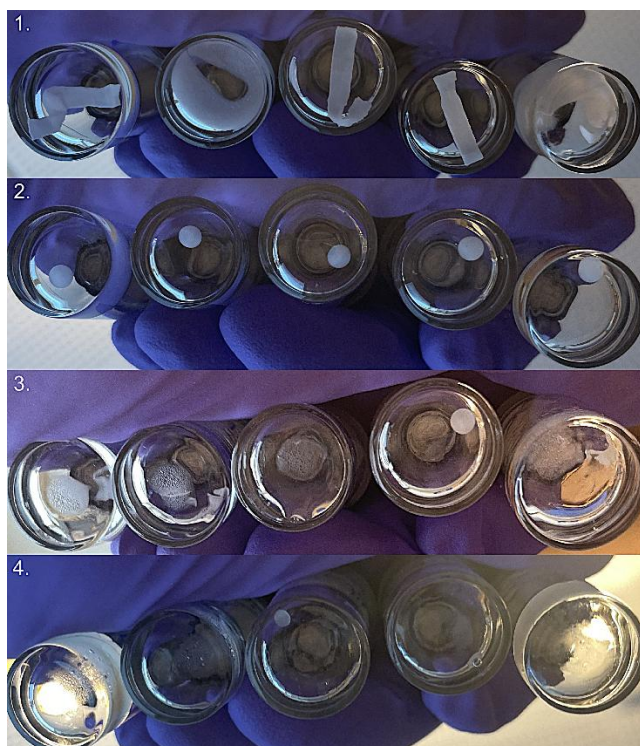
Figure 16. Gradual degradation of control-A-PLGA samples by rows.
