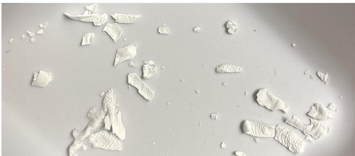
Figure 18. Broken control-B-PLGA samples after removal from PBS.
