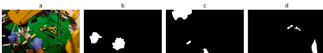
Fig. 12. (a) an OOD data of two human operators O2 with gloves (GH) having rare gestures (RG) in the egocentric view, (b) the segmentation ground truth mask, (c) segmented by DE-Mix trained on EgoHands, (d) segmented by DE-Mix trained on Ego2Hands.
