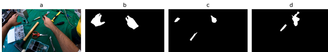
Fig. 10. (a) an ID data in the egocentric view, (b) the segmentation ground truth mask, (c) segmented by DE-Mix trained on EgoHands, (d) segmented by DE-Mix trained on Ego2Hands.
