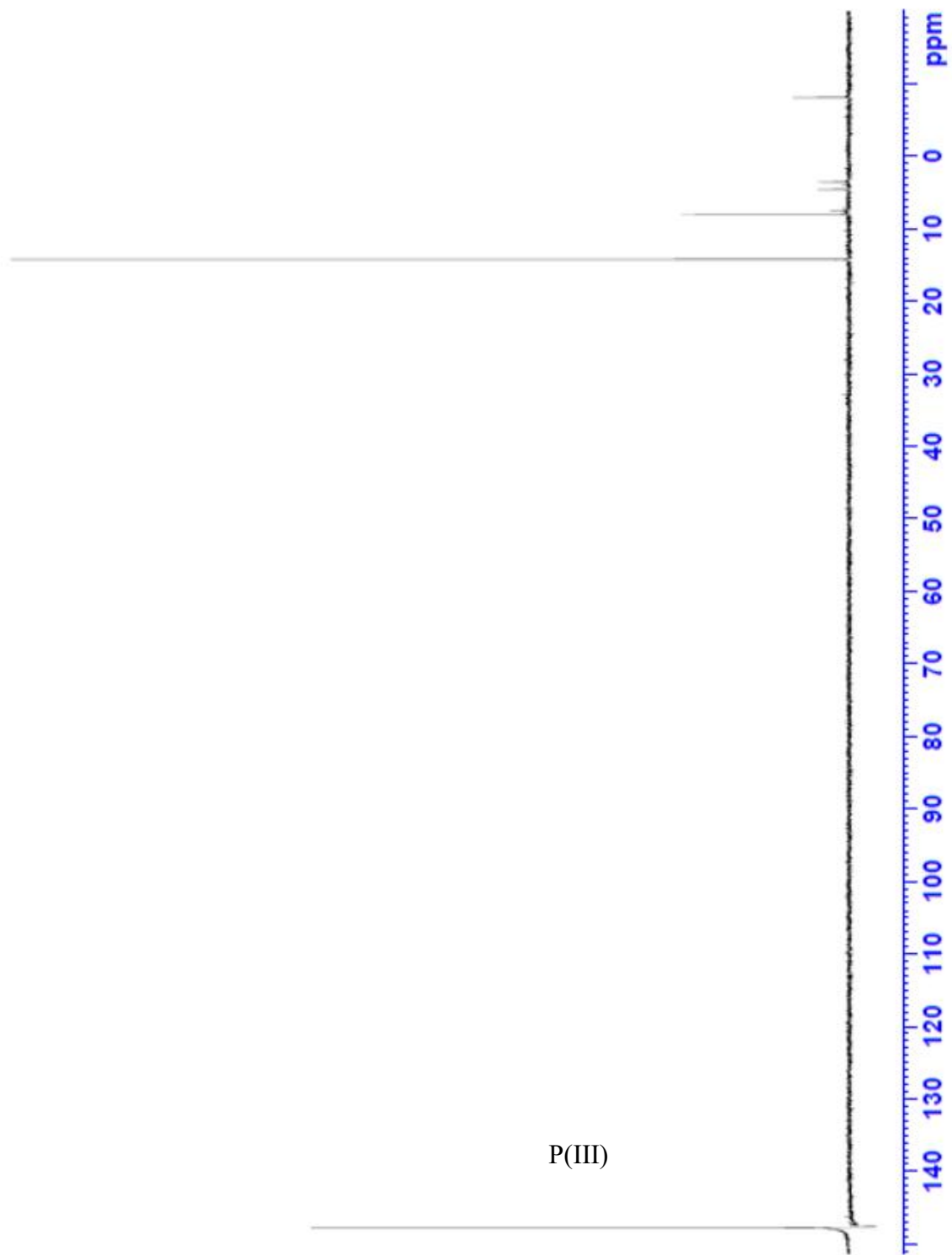
Figure 19 ^{31}\text{P} NMR spectrum of phosphoramidite 8
