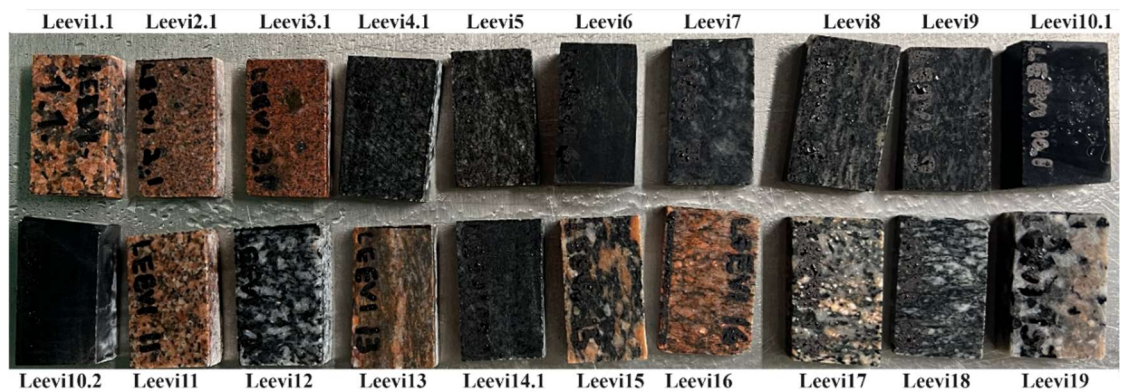
Figure 7. Rock samples after cutting. Size of the cutted samples is 3.5 x 2.5 mm.
