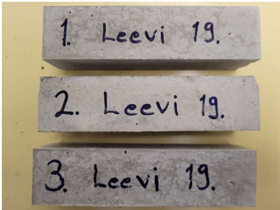
Figure 9. Example picture of prepared mortar bars from rock sample Leevi19.
