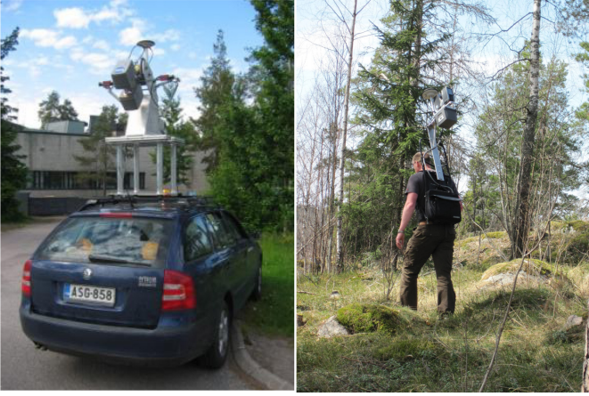
Fig. 3. MLS platforms used to gather the data. (Left) Vehicle mount for built environment. (Right) Backpack mount for forest.
