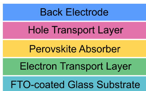
Figure 1. Scheme of a conventional perovskite solar cell, FTO – fluorine-doped tin oxide.
