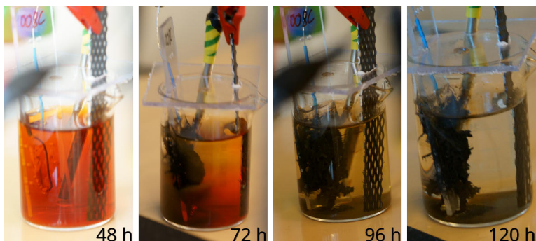
Figure 29. Pd-D co-deposition cell (PdE-008C) at different times over the experimental period. At higher currents, corresponding to higher applied potentials, the dissolved palladium deposits on the Ag working electrode dendritically and grows toward the counter electrode. Bubbles created by the gas evolution reactions disrupted the dendritic growth of the palladium deposit breaking parts of the deposit off, which proceeded to precipitate at bottom of the cell. Figure from Publication II .
