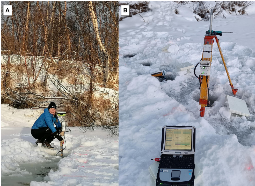
Figure 8. Two ADCP measurement setups are used to collect data beneath the ice. In the first, the ADCP (SonTek M9) device is handheld by the researcher (A), and in the second, it is attached to a tripod (B).
