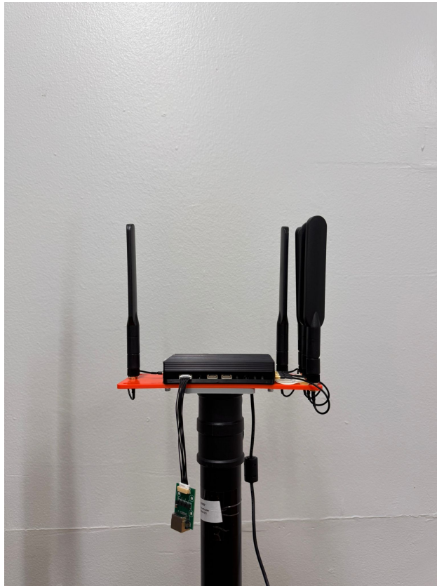
Figure 3.4: Robonode-M mesh module used as a Linux-based mesh node, integrated directly on the robotic platforms via Ethernet.
