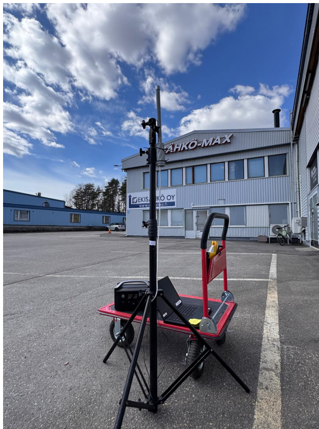
Figure 3.3: MikroTik Groove A52 radio used as a mesh node. The unit is powered over passive PoE and carries an integrated dual-band antenna.
