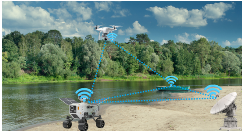
Figure 1.1: Unmanned Aerial Vehicles (UAVs), Unmanned Surface Vehicles (USVs), and Unmanned Ground Vehicles (UGVs) are working cooperatively as a MRS to monitor a riverine environment © 2026 IEEE
