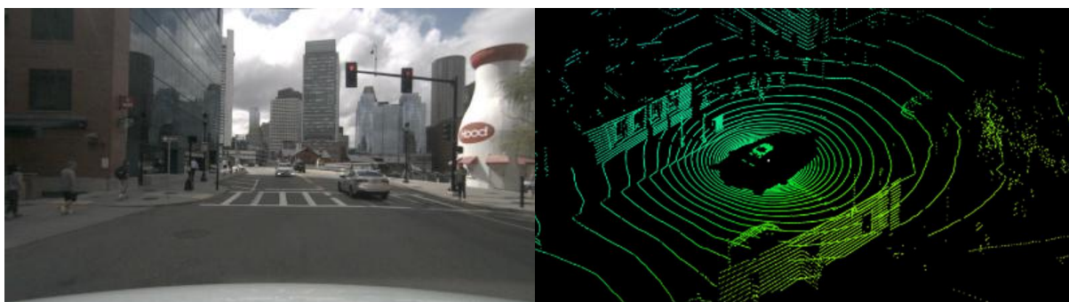
Figure 2: Camera image (left) and LiDAR point cloud (right), modified from [4] © IEEE (2024)
