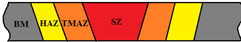
Figure 2. Formed material zones in FSW
