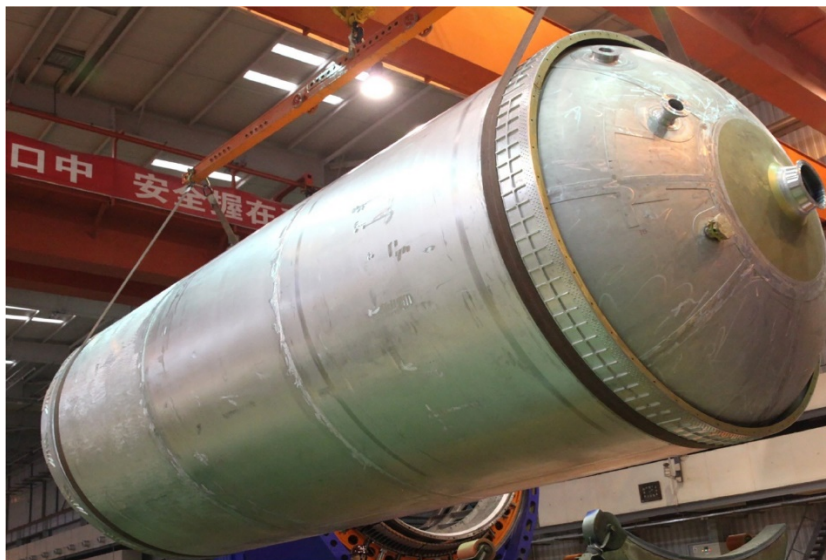
Figure 6. Application of FSW on a rocket tank. Reprinted from Journal of Materials Science & Technology , Vol 34/1, Guoqing Wang, Yanhua Zhao, Yunfei Hao, Friction stir welding of high-strength aerospace aluminum alloy and application in rocket tank manufacturing , pages 73-91, Copyright 2018, with permission from Elsevier. [20]
