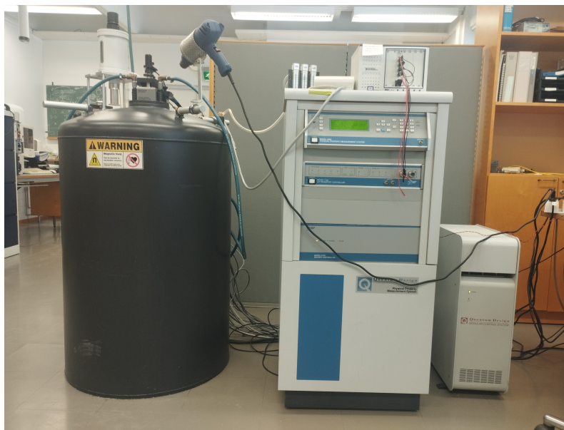
Figure 4: PPMS utilized in this study highlighting the sample chamber, temperature control and measurement probes essential for assessing the magnetic properties of samples across a broad temperature and magnetic field range.
