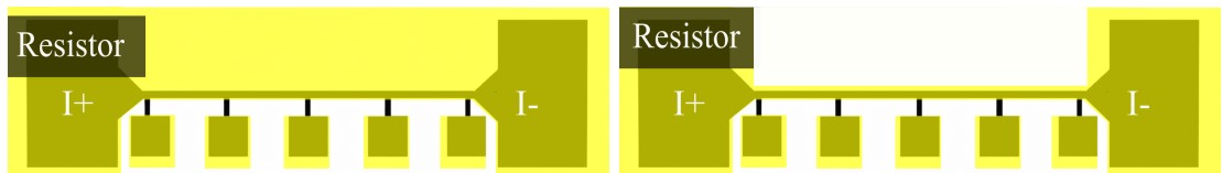
Figure 8: Illustration of a stripes fully (left) and narrowly (right) coated with Au, where the spacing between adjacent channels is 1 mm.
