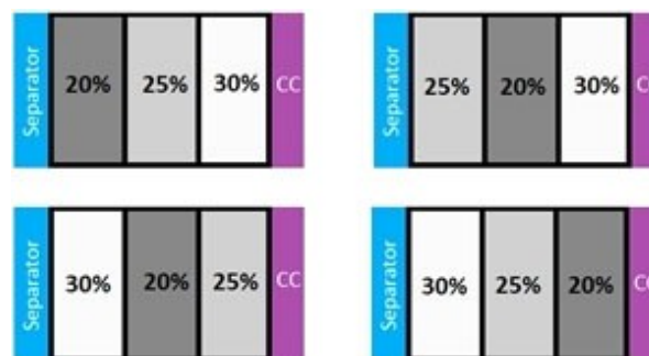
Figure 13. The porosity heterogeneities in the four types of cathodes. The electrodes are composed of three layers placed between the separator and the current collector (CC).
