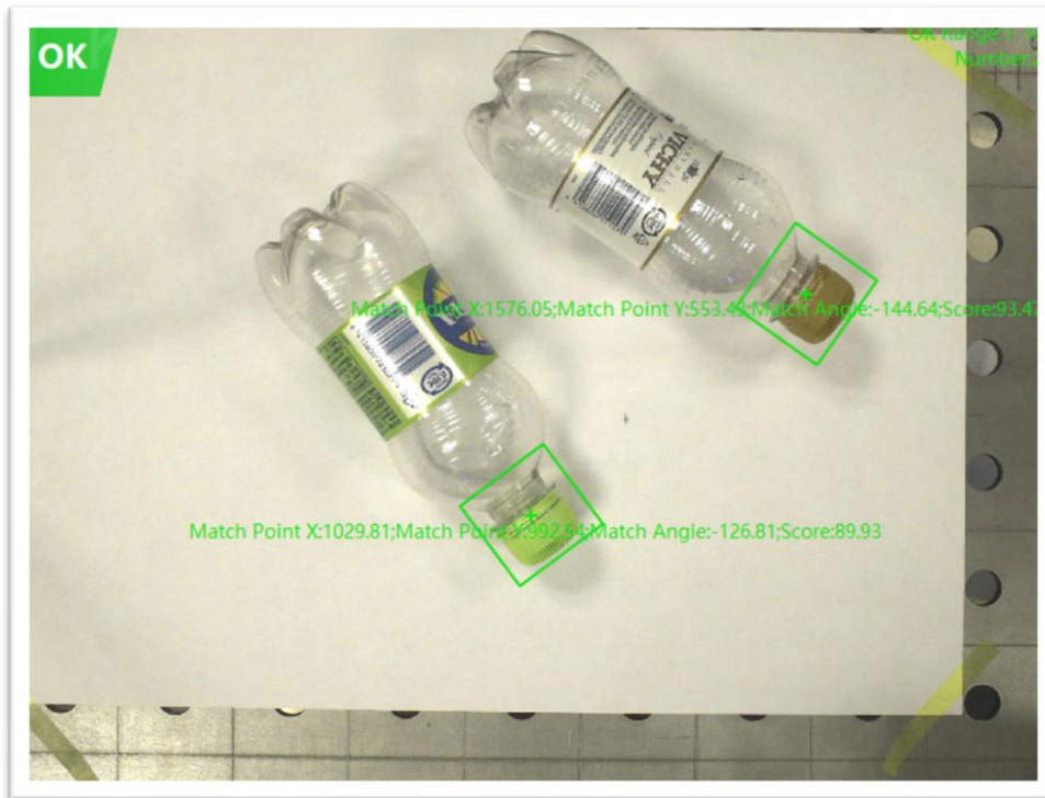
Figure 8. Experiment with translucent water bottles showing successful detection of two target objects through training the feature template for finding the bottle caps. Screenshot from Hikrobot SCMVS - software, Veeti Suominen, 2026.
