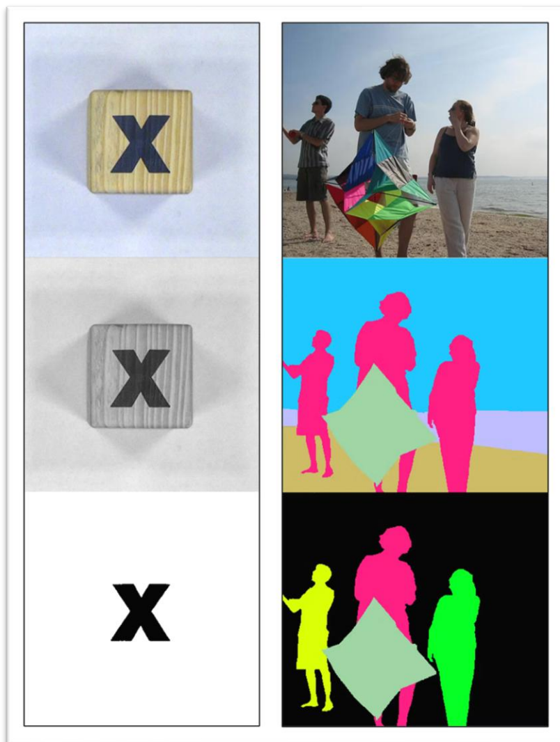
Figure 2. Left side shows the simplified steps of threshold image segmentation. The right side shows the simplified steps of semantic- and instance image segmentation. Left image: Veeti Suominen, 2026. Right image: edited from https://encord.com/blog/guide-to-semantic-segmentation/ , Nikolaj Buhl, 2024.
