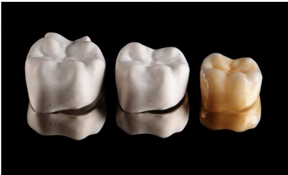
Figure 8. 3D printed dental crowns made of zirconia. Green body (right), after debinding (centre) and final sintered part (left). Reproduced from ref. [19].
