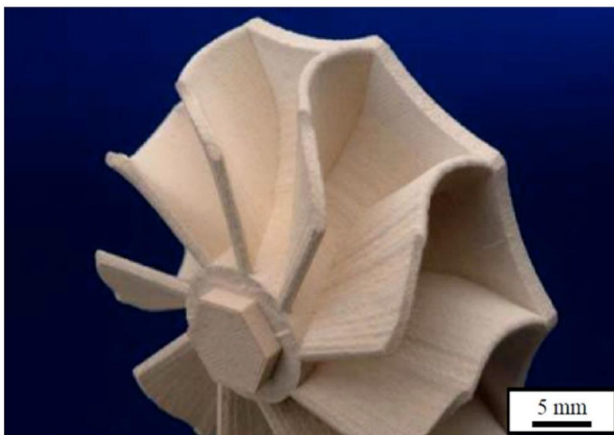
Figure 9. Turbine of a turbocharger made with SLM out of 80% zirconia / 20% alumina. Reproduced with permission from ref. [22]. Copyright 2013, Emerald Group Publishing Limited.
