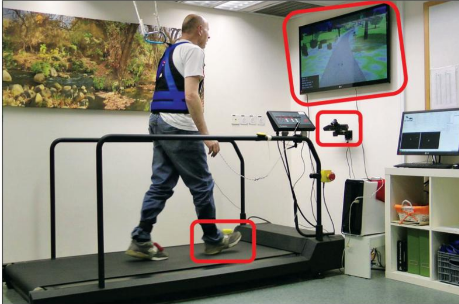
Figure 2. Treadmill + Virtual Reality training set-up. From Mirelman et al. (Mirelman et al., 2016)- V-TIME project
