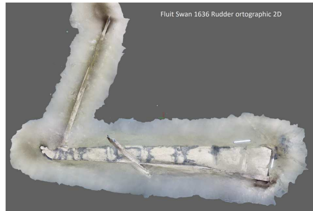
Figure 11. 3D model of the rudder with its still-attached tiller. Rudder is 8.3 m measured along the line of sternpost from the keel up to the trefoil carving on the top. The tiller is 5.0 m long (Jouni Polkko/Badewanne).
