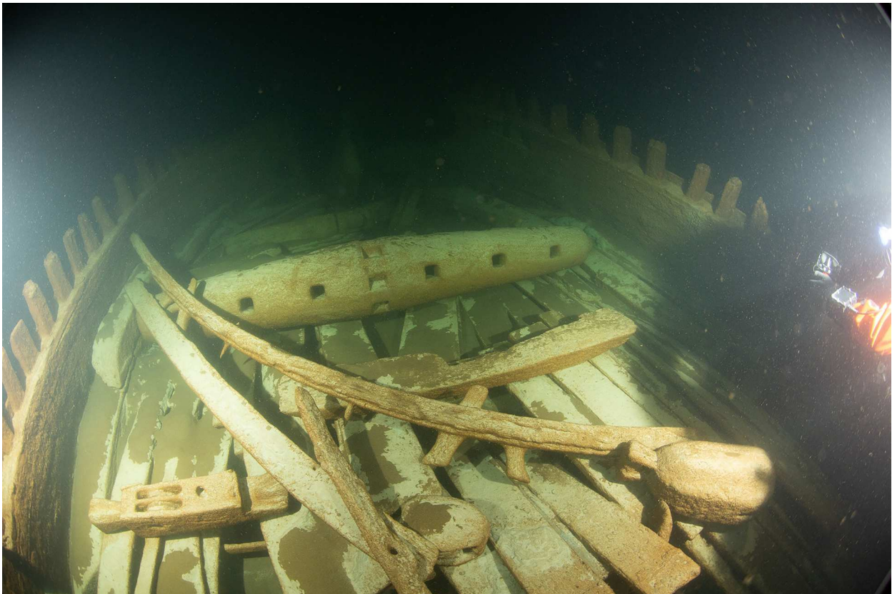
Figure 7. The windlass has moved slightly out of place. Note the beam with the pinrail and kevels as well as the knight (to the left) and an anchor buoy to the right (Jouni Polkko/Badewanne).
