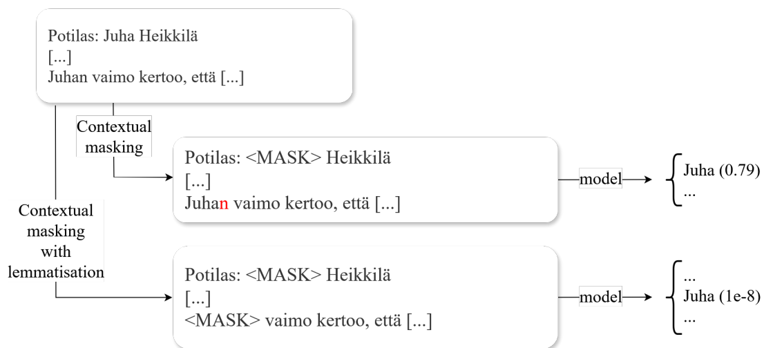
Figure 5.3: Figure illustrating the problem with Finnish conjugations. The example translates to “Patient: Juha Heikkilä [...] Juha’s wife says that [...]” with the possessive suffix that prevents regular contextual masking highlighted in red. Masking the tokens that make up the word “Juha” might not mask the word “Juhan” as it might not comprise the same tokens as “Juha”. With internal lemmatisation, the masking is done correctly.
