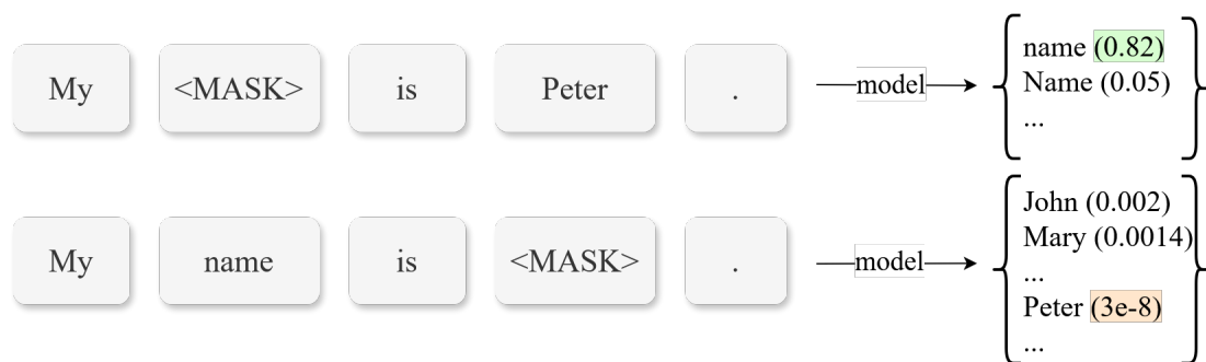
Figure 4.1: Illustration of the zero-shot PII redaction method. The model can easily predict the masked word “name”; however, it struggles to predict the word “Peter”, resulting in weak guesses overall. The probability value of Peter is low, which means that “Peter” cannot be inferred from the context and is likely PII.
