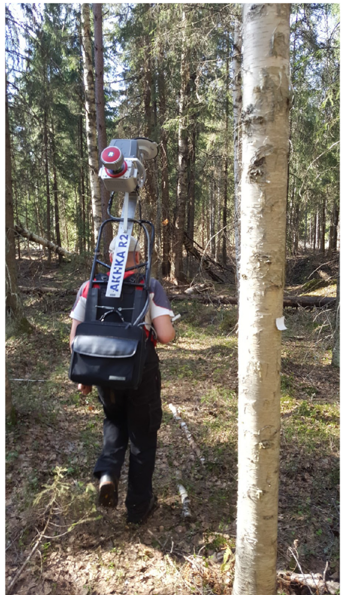
Fig. 1. Applied Akhka-R3 backpack laser scanner instrument scans 360-degree cross track profiles while GNSS-IMU tracks the platform dynamics during the kinematic mapping.
