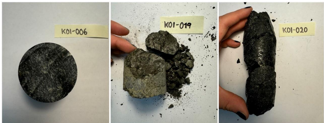
Figure 15. Three representative drill core samples from the Koillismaa deep Hole between depths of 1,500–1,700 m. KOI-006 (left) and KOI-020 (right) are classified as altered peridotites. Sample KOI-019 (middle) differs from the ultramafic lithologies and is characterized by a fractured mafic mineral assemblage with subordinate felsic components.
