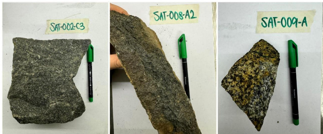
Figure 14. Three diabase samples gathered around Satakunta, SW Finland. Massive, homogeneous relatively unaltered and equigranular diabase samples from Olkiluodontie, Eurajoki (SAT-002-C3) and Makholma (SAT-008-A2), as well as coarse-grained diabase sample from Mäntykallio (SAT-009-A).
