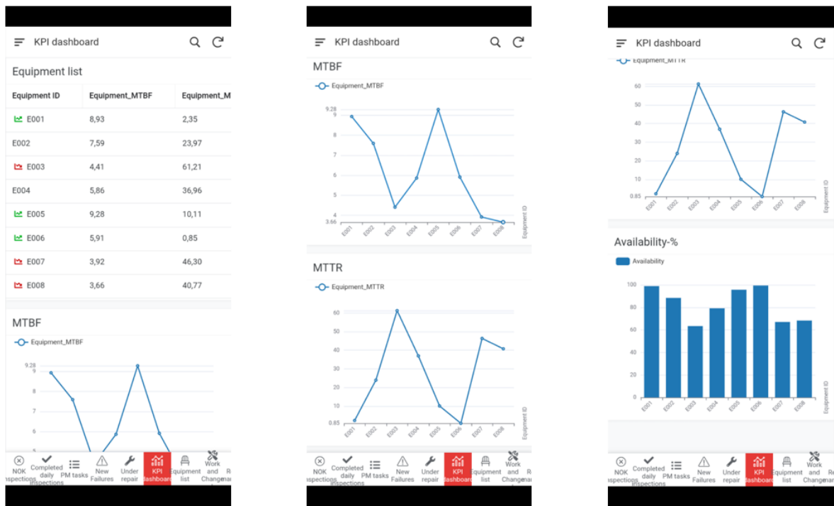
Figure 45 - The KPI dashboard displaying equipment failure rates and efficiency, providing live status for management.
