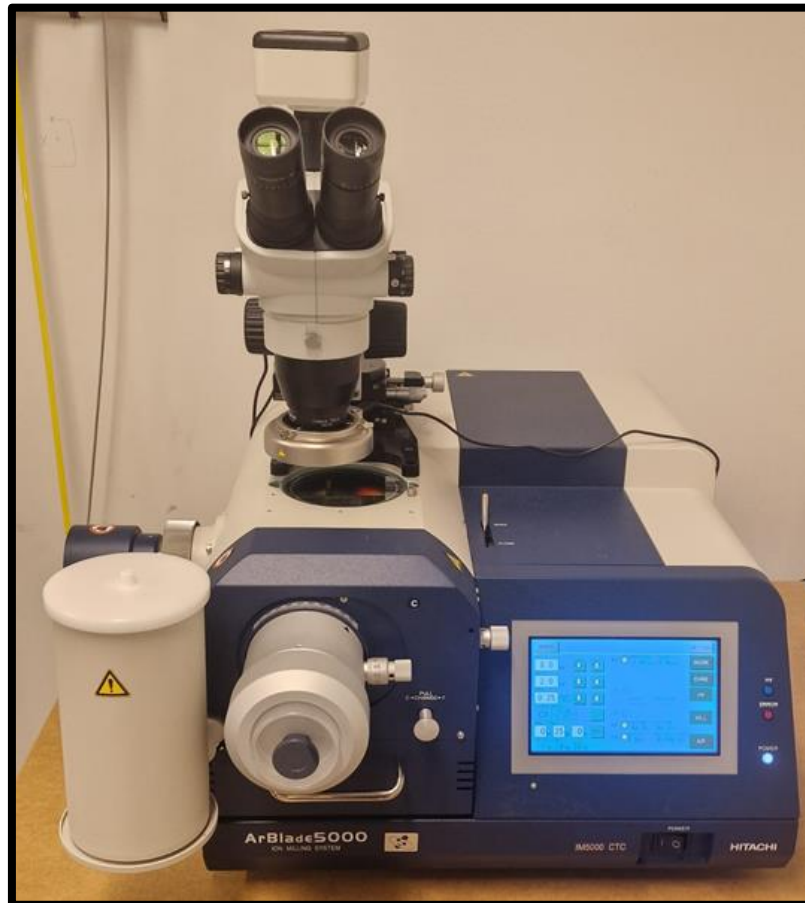
Figure 10 shows image of Ion Milling Setup (ArBlade 5000, Hitachi High-Technologies) available in Quantum building, University of Turku.
