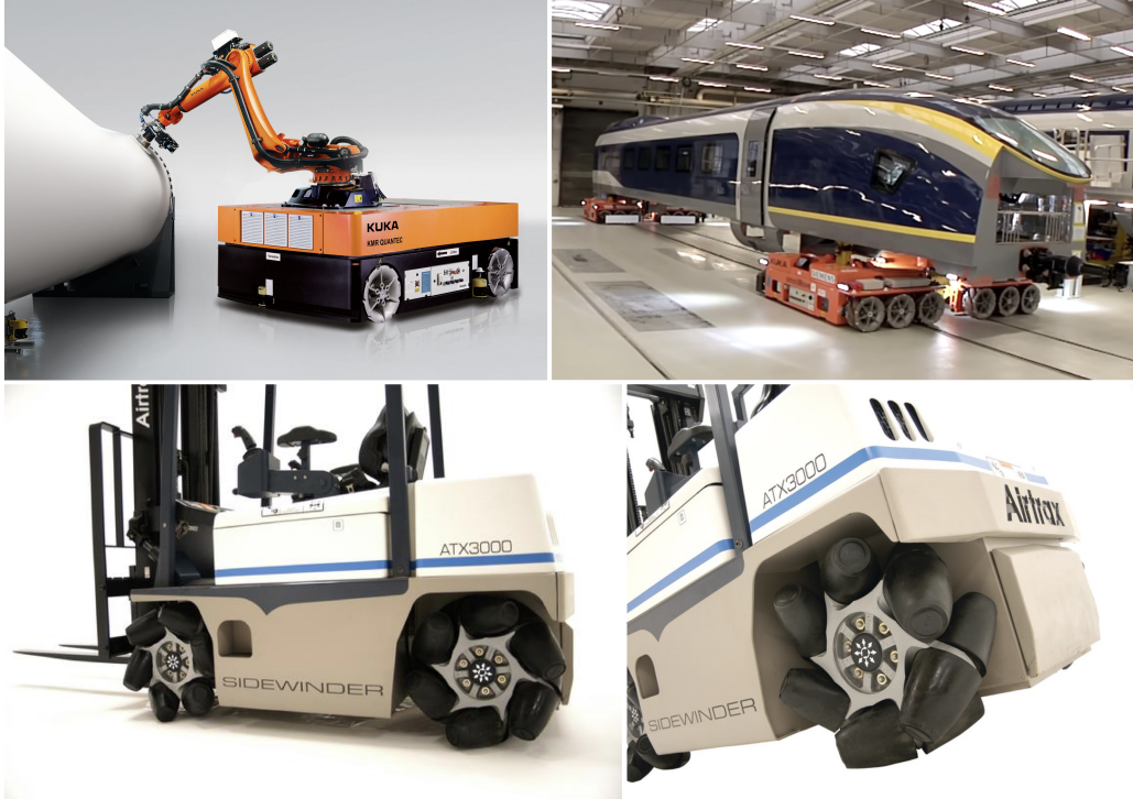
Figure 1.3: Some applications of Mecanum-wheeled platforms. Top left: KUKA KMR QUANTEC AGV in aerospace manufacturing. Top right: Mecanum-wheeled transporters positioning a train body in an assembly hall. Bottom: Airtrax ATX3000 Sidewinder omnidirectional forklift. Source: Moreno Caireta (2019).
