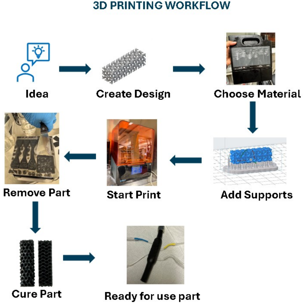
Figure 1.1: Schematic representation of the stereolithography (SLA) 3D printing workflow used in this study.
