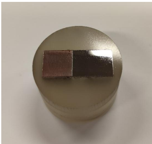
Figure 33 Sample set in acrylic compound.
