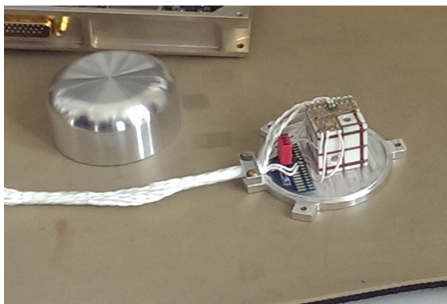
Fig. 3. The IWF MAG flux gate magnetometer head.
