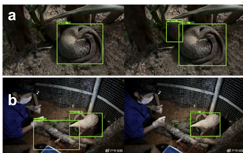
Fig. 3. Examples of images where the Faster R-CNN ResNet101 with MS COCO weights failed to design and predict the pangolins object detection boxes (left images – detected boxes; right images – real boxes). (a) with more than one pangolin and displaying additional pangolin parts; (b) presenting dark colours and emphasized shadows. The sources of the images displayed in this figure are referred in the supplementary material.
