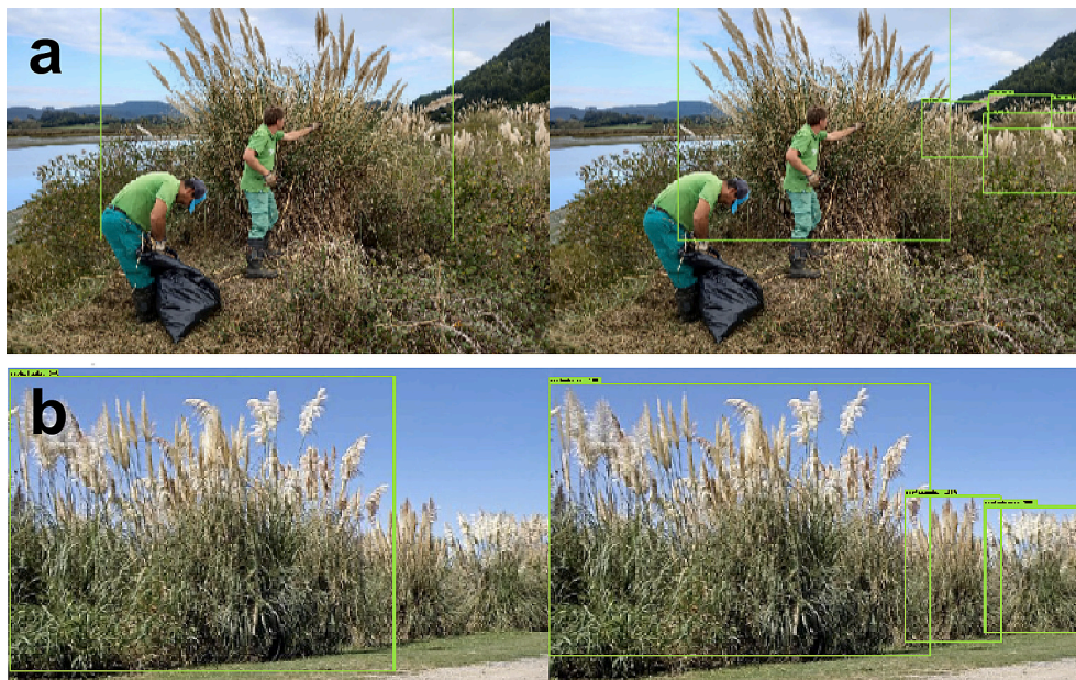
Fig. 4. Examples of images where the Faster R-CNN ResNet50 with MS COCO weights failed to design and predict Cortaderia selloana object detection boxes (left images – detected boxes; right images – real boxes). (a) with C. selloana in the background, reduced in size or barely visible; (b) with more than one C. selloana .
