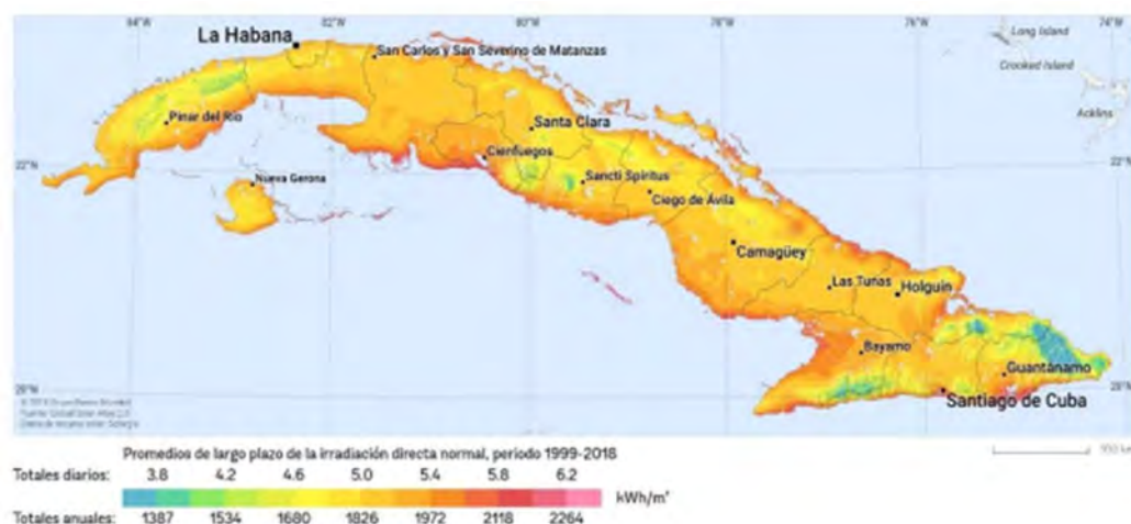
Figure 2. Map of average normal direct irradiation in Cuba, period 1999 – 2018 (Solargis, 2021).
