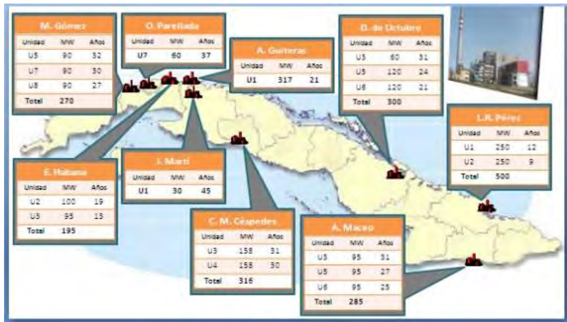
Figure 2. Installed capacity in the NEES for 2004 (UNE, 2004).
