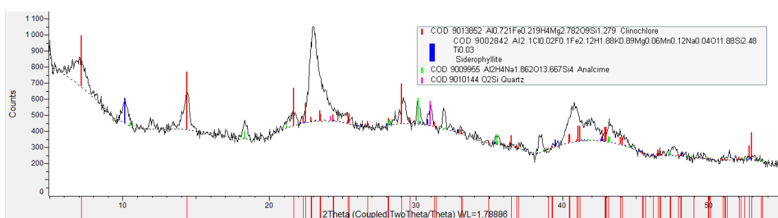
Figure 56. Diffractogram of the sample MM196_98_35. It was very challenging to match logical minerals to most of the peaks. The peak profile is somewhat messy.
