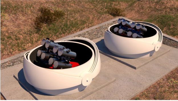
Figure 16. Visualization of a full GOTO node site consisting of 16 UTs spread over 2 domes. The northern and southern nodes will contain identical sets of 2 \times 8 , providing a total of 32 UTs.
