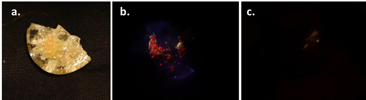
Figure 36. DDM glass sample doped with MGO:Cr 19% : a. under room lighting; b. under electron beam excitation; c. PeL after electron beam excitation.
