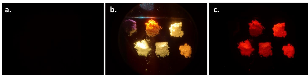
Figure 7. Photographs of samples MgO, MgO:Ce 0.12% Sm 0.12% , MgO:Li 6% Ce 0.06% Sm 0.06% , MgO:Li 12% Ce 0.12% Sm 0.24% , MgO:Li 9% Ce 0.06% Sm 0.06% , and MgO:Li 3% Ce 0.06% Sm 0.06% (listed from left to right, top to bottom): a. in the darkness, b. under a 12.5 keV electron beam excitation, c. after the electron beam is turned off.
