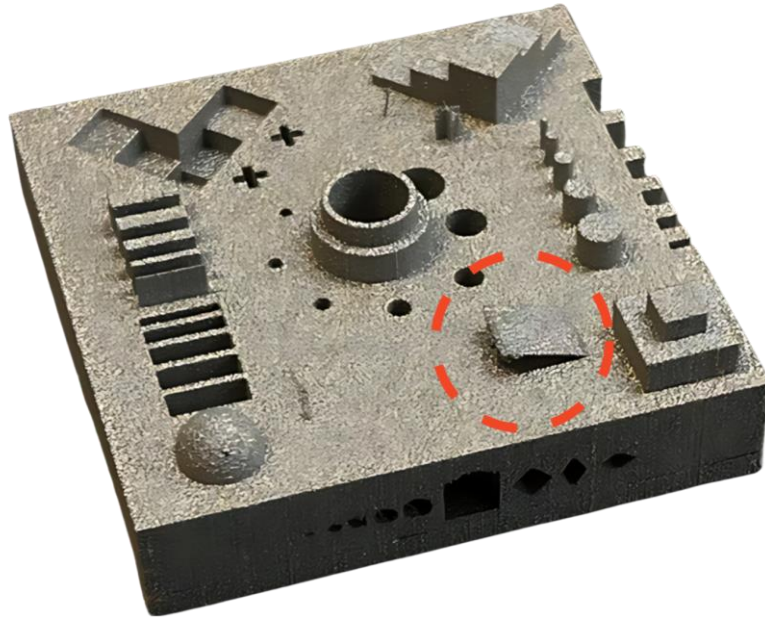
Figure 21: The first AMed artifact on Aconity3D MIDI+ appears to be a failed attempt to make the inclination surface used to assess the overhangs.
