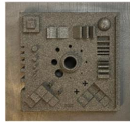
Figure 26: Single Benchmark artifact labeled sample 2 AMed on a build plate of Aconity3D MIDI+.
