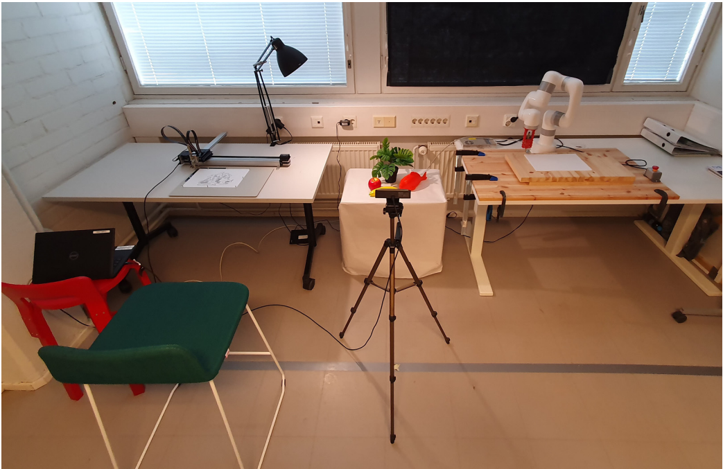
Fig. 5. Experimental setup including the robots (AxiDraw, left; xArm), arrangement, camera and participant chair. Missing from the picture is the folding screen, which was initially used to keep the robots out of sight.
