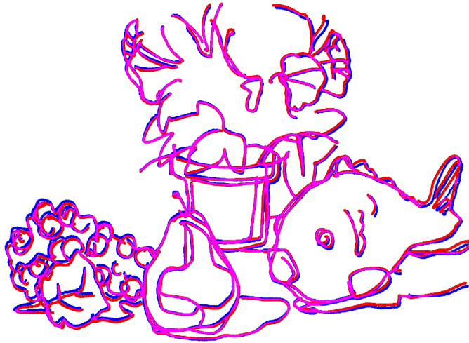
Fig. C1. Example of the differences in overlaid drawings produced by AxiDraw (pink) and xArm (blue).
