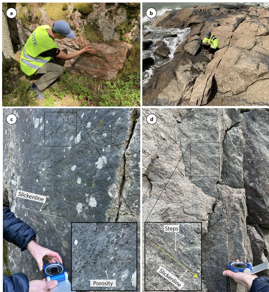
Fig. 3 Field mapping of fault zones in the Vehmaa Batholith. a Strike-slip fault associated with mineral alteration marked by the reddish coloration . b Example of a joint network with multiple orientations. c A SE-striking fault plane associated with a weak sub-horizontal fault lineation and observable secondary porosity. d A S-striking fault plane with well-marked oblique slickenlines. The fault surface also exhibits steps, which are useful for determining the sense of slip (slickenline orientation and the dextral sense of movement on the fault surface are visualized with the yellow arrow ). In both images c and d , the compass lid and body edge trends to the south
