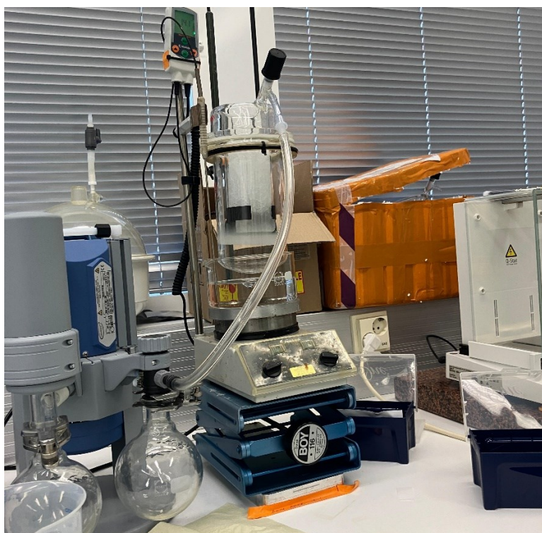
Image 2: Sublimiter to apply DHB matrix onto brain tissue slices.
