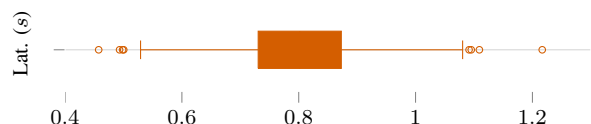
Fig. 7: Latency distribution for a simulation of three drones following the three trajectories in Fig. 6.
