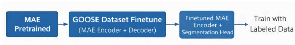
Figure 4.2: Two-stage training pipeline: domain-adaptive MAE pretraining followed by supervised fine-tuning.
