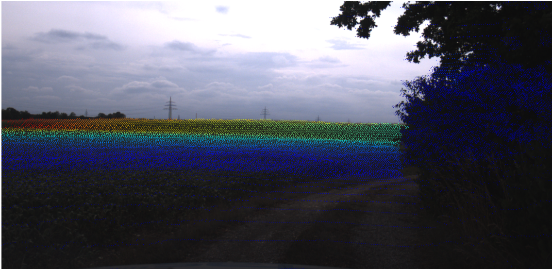
Figure 3.2: LiDAR Depth Point Cloud Overlay on Image, Highlighting Increased Point Density in the Horizontal Center Crop, Different depths are shown in different colours.
