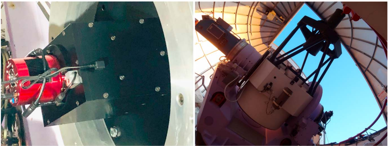
Figure 1. Left: DIPOL-1 polarimeter with its CMOS camera on the T90. Right: T90 telescope. Credit: IAA-CSIC.
