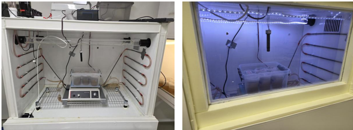
Figure 16. Setup for the lighting experiment. Light treatment cultured inside a growth box with 12 h of light.
