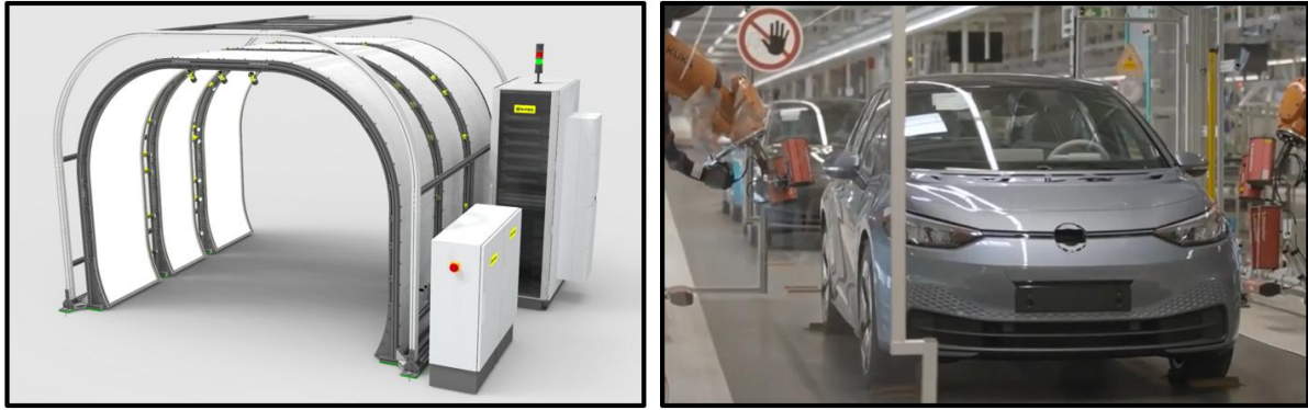
Figure 14. Machine vision panel gap and flush inspection solutions from suppliers, with the machine vision tunnel from Eines Vision on the left and machine vision robot station from Isra Vision on the right. From: [31, 32].
