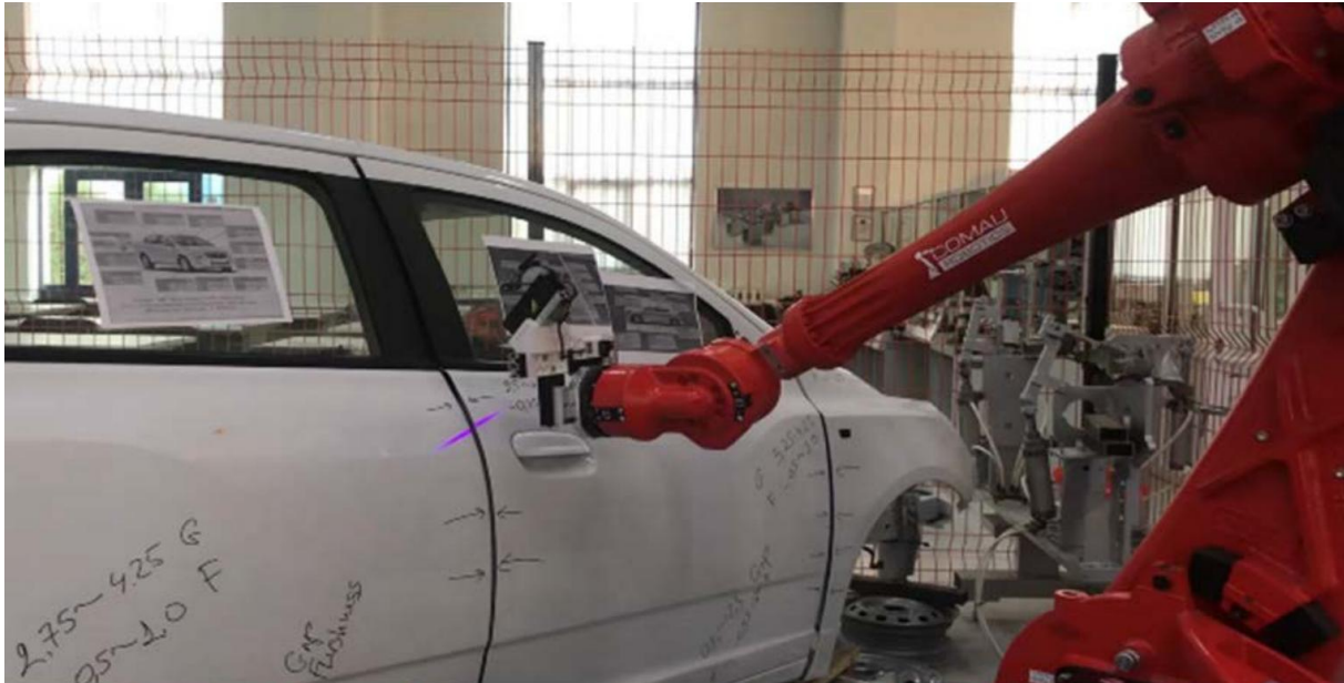
Figure 13. Robotic panel gap and flush inspection setup. From: Kholkhujaev et al. [30].
