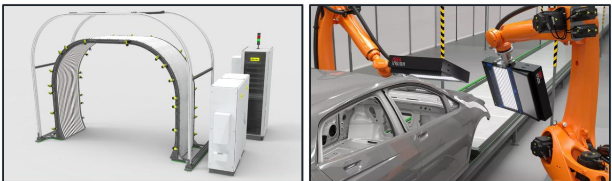
Figure 11. Machine vision paint inspection solutions from suppliers, with the machine vision tunnel from Eines Vision on the left and machine vision robot station from Isra Vision on the right. From: [26, 27].
