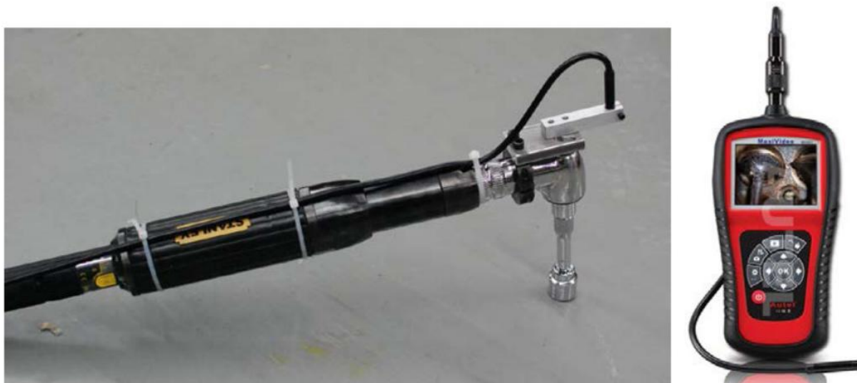
Figure 4. Autel MV201 video inspection camera mounted on a fastener tool. From: Rusli and Luscher [33].
