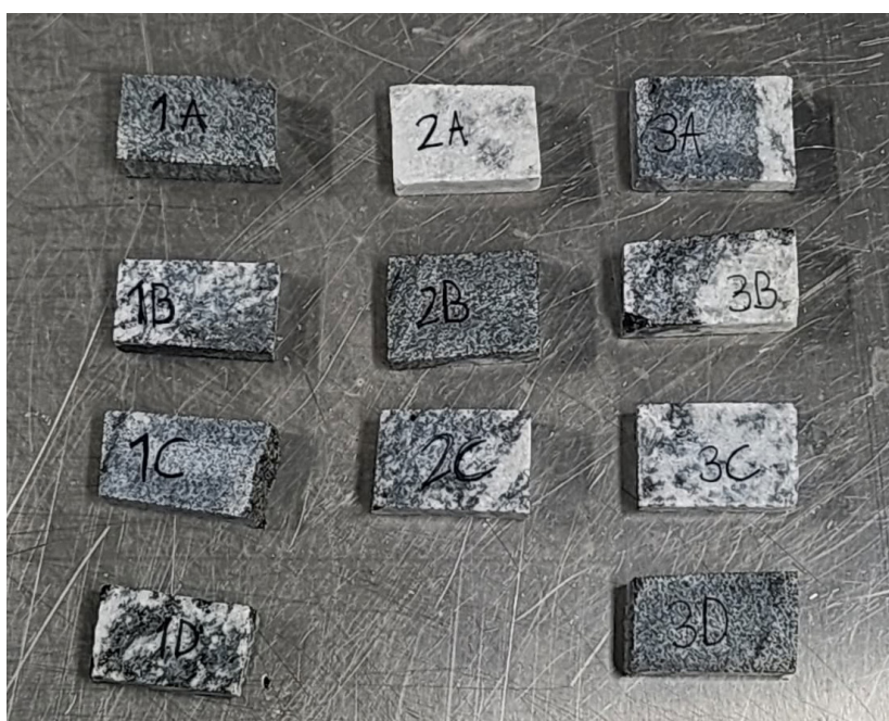
Fig. 8: The sawed rock pieces used to make thin sections.
