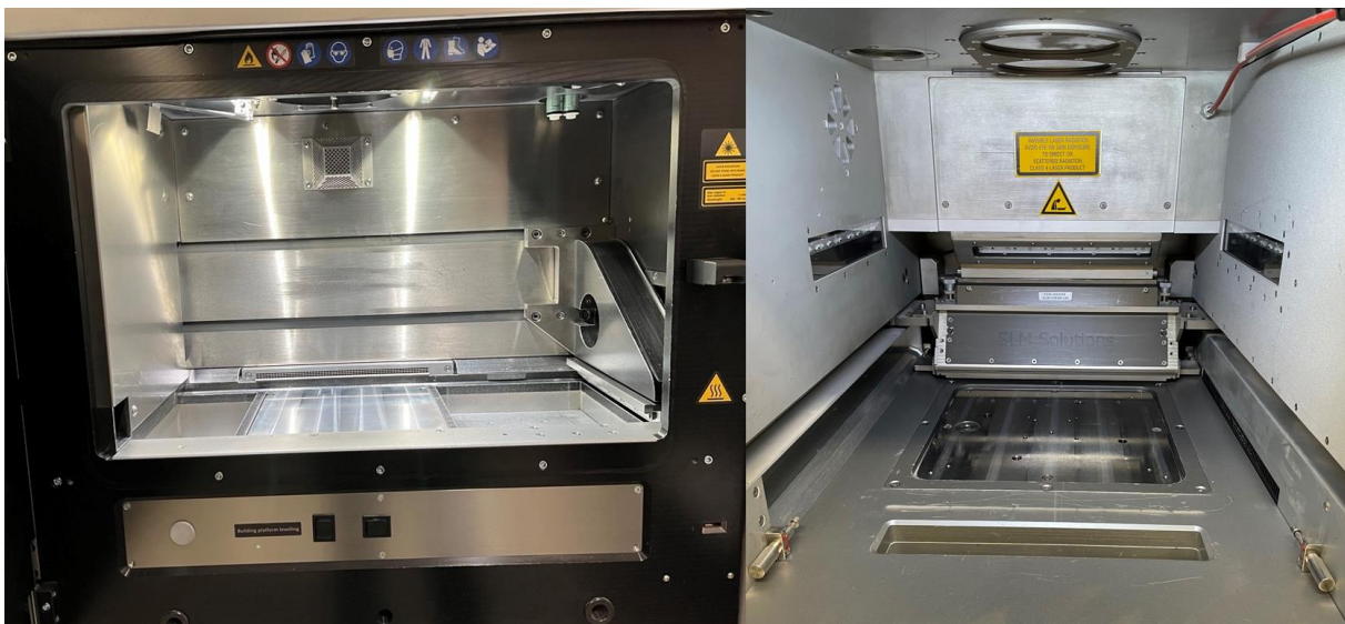
Figure 4 Side-by-side pictures of M290 building chamber on the left and 280HL on the right
