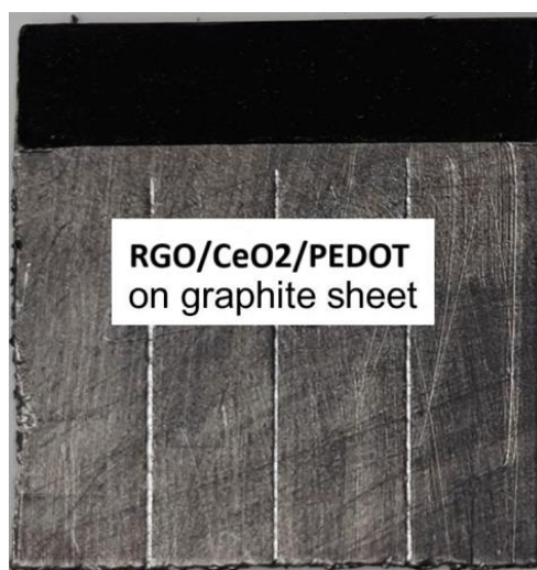
Figure 15 RGO/CeO 2 /PEDOT loaded electrode.
