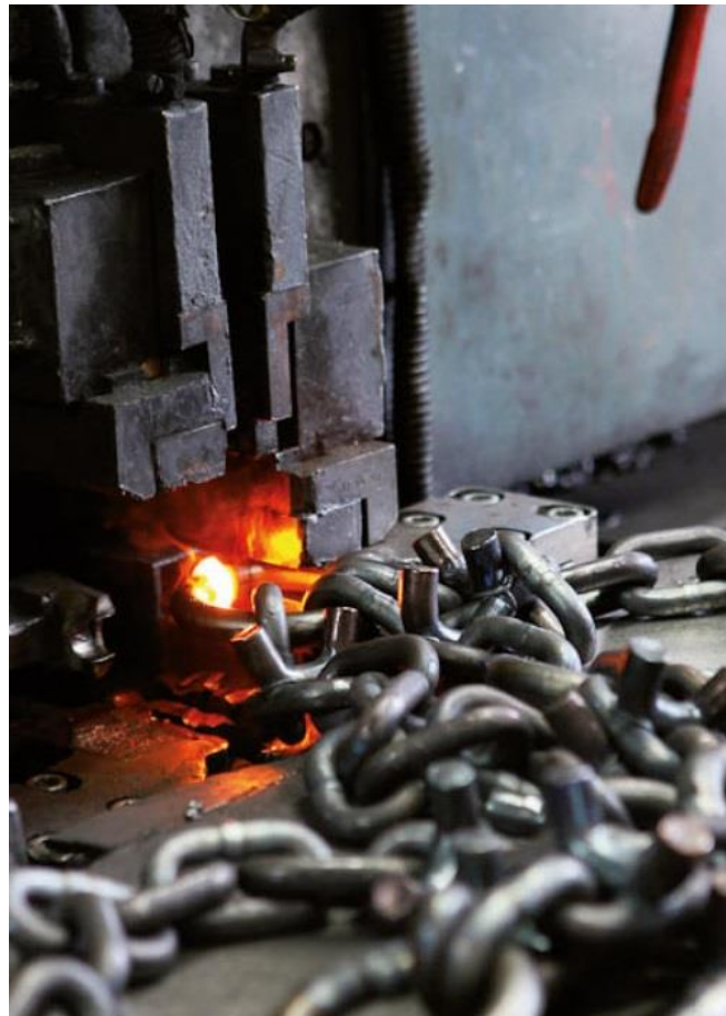
Figure 1. Boron steel chains being heated and pressured together in high pressure. Image reproduced with permission from [1].
