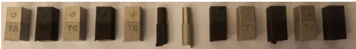
Figure 33. A photograph of all twelve workpieces from the second test batch. The workpieces are set from designation "TA" to "TL", in alphabetical order, from left to right. Every other workpiece is heat-treated, and has undergone notable oxidization on the surface during the heat treatment. The two middle parts were the workpieces meant for dilatometry tests, which fell out of the scope of this thesis.
