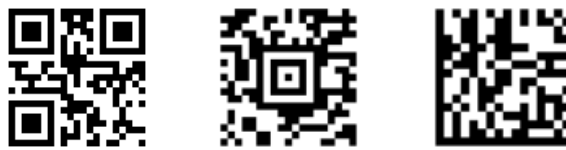
Figure 2.1: Examples of a QR code, an Aztec code and a Data matrix [9]. All containing the message "Example Code".
