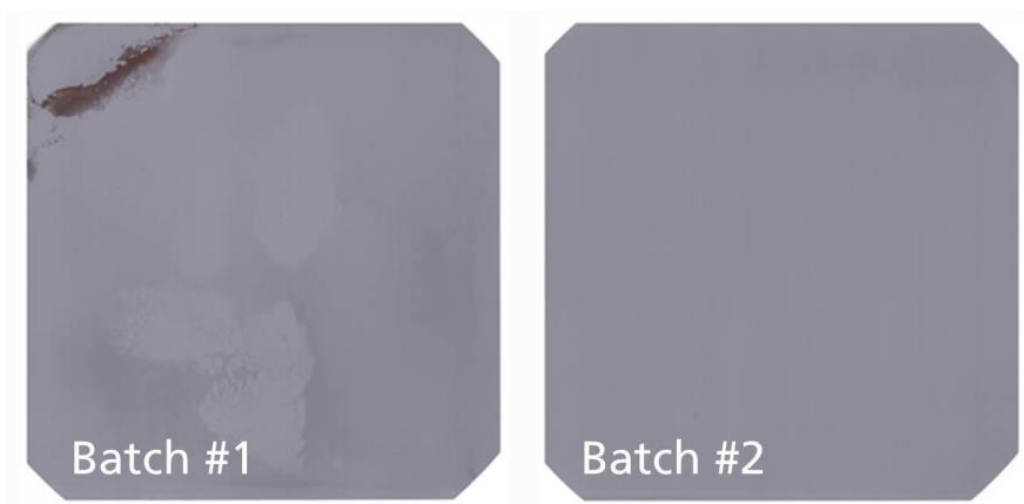
Figure 10: Batch 1 pre-cleaned by water and batch#2 by NaOH/IPA [16]
