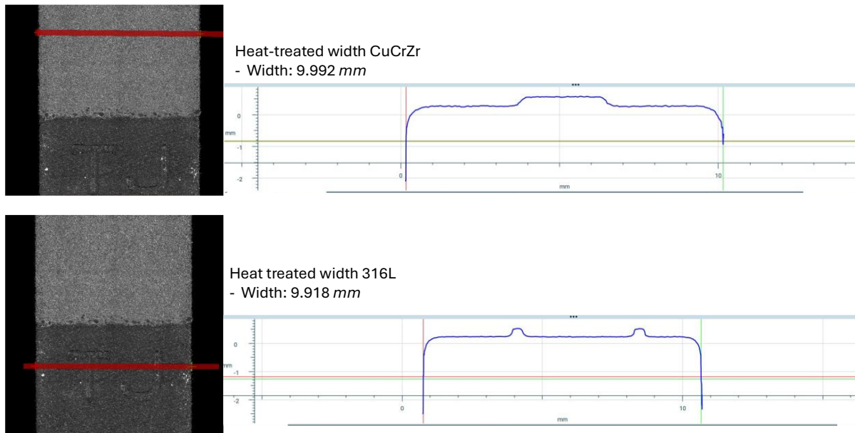
Figure 34. Geometrical accuracy measurements of the widths of the HT1 CuCrZr and 316L (left top and left bottom), and corresponding line graphs showing the scanned profiles and measured width values (right top and right bottom).
